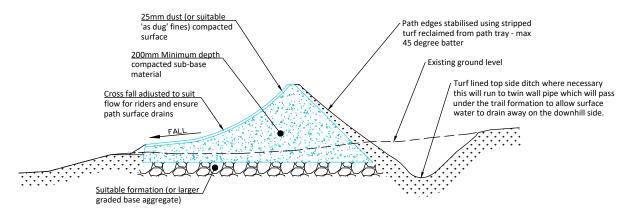
**Typical 'Berm' Trail Construction Detail**
