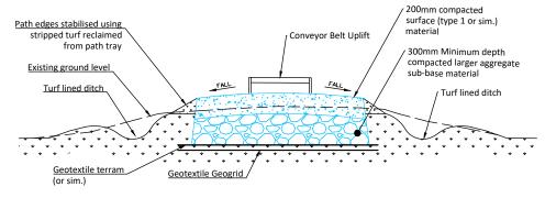
**Conveyor Belt Track Construction Detail**
