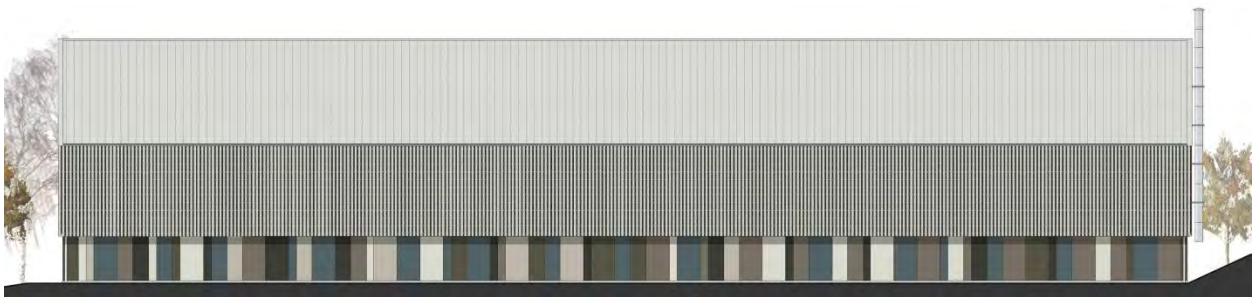
Fig 12. Render replaced with rainscreen cladding to harmonise with remainder of the building.
