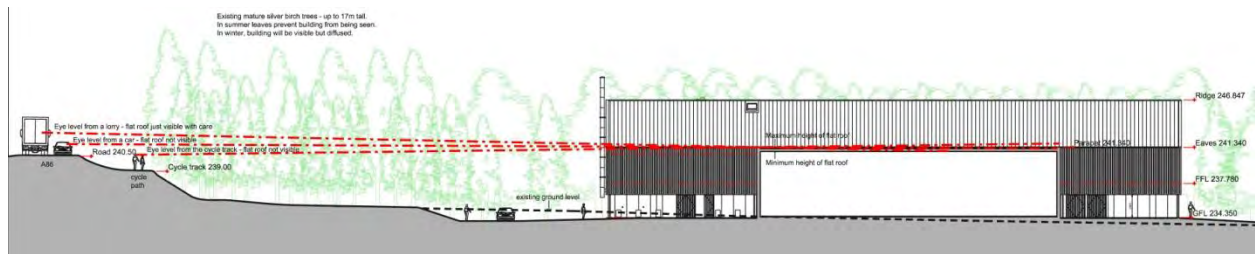
Fig. 4 Section through flat roof showing viewing lines of visibility from the A86 and cycle path.
