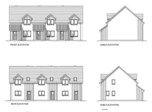
Type 2B4PV – two bedroom terraced one and a half storey houses (three in terrace)
