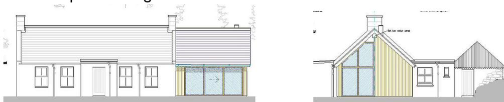
Fig. 6 : Keeper's Cottage extension (front and side elevation)
