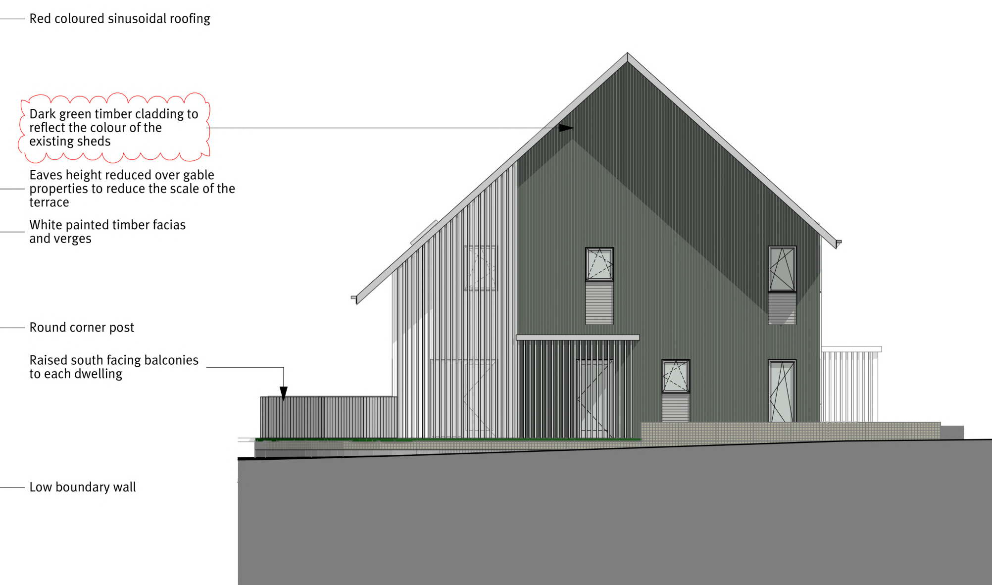
E12 Block C East Elevation 1:100
