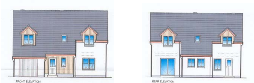
Fig. 6 : House type A – Front and rear elevations
