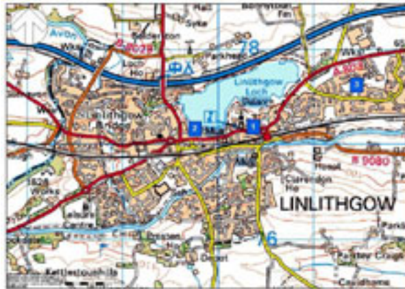
Figure G1.5 The plans of many Scottish villages, towns and cities illustrate different patterns of development over time, from (1) historic cores, through to (2) experimental 'Radburn' layouts from the 1960s, to (3) recent cul-de-sac layouts.
