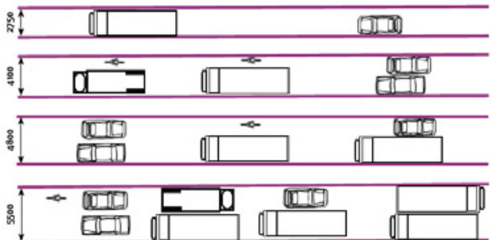
Figure G4.1 Illustrates what various carriageway widths can accommodate. They are not necessarily recommendations.
