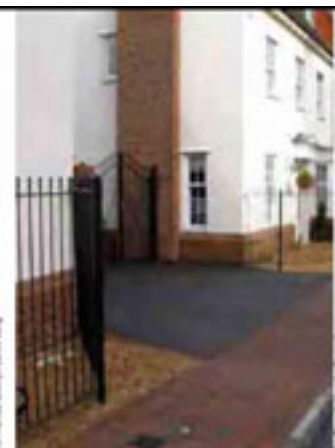
Figure G4.21 Beaulieu Park, Chelmsford: the visibility splays are provided by railings rather than boundary walls, although the railings could have followed the property boundary.
