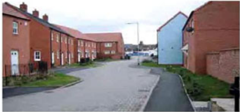
Figure G4.13 This street avoids the use of vertical traffic-calming features, but the irregular alignment is unsightly and unlikely to have much speed-reducing effect, because of the width of the carriageway. It also results in irregular grassed areas that create a maintenance burden while contributing little to street quality.
