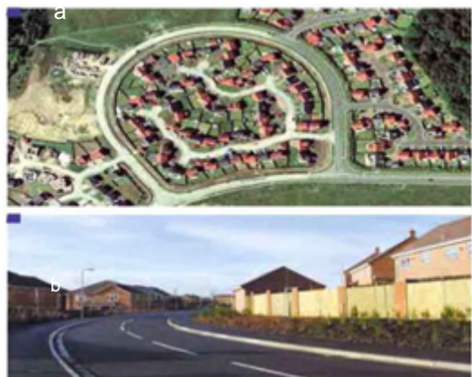
Figure G2.7 (a) and (b) Cul-de-sacs surrounded by a perimeter road that is fronted by back fences - no sense of place, no relationship with its surroundings, no quality, with streets designed purely for vehicles
