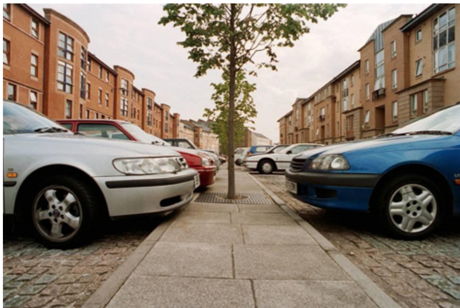
Figure G5.9 An example of on-street parking in the centre of the street in Glasgow that helps to separate the car from other users and provides strong surveillance of the cars (Scottish Government).
