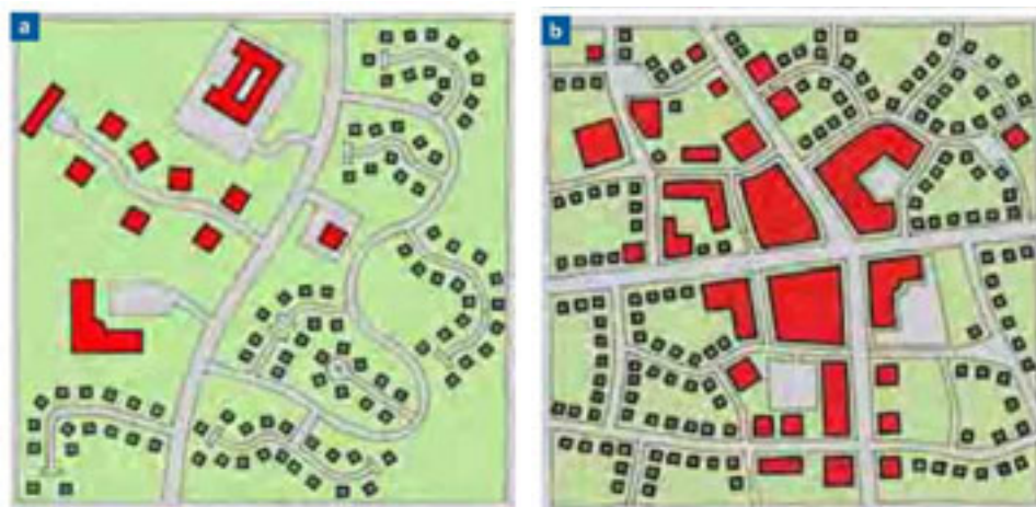
Figure G1.4 (a) dispersed and car-dependent versus (b) traditional, compact and walkable layout
