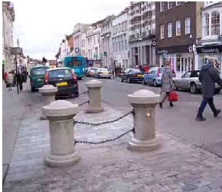
Figure G3.2 Informal crossing, Colchester - although the chains and a lack of tactile paving are hazardous to blind or partially-sighted people.
