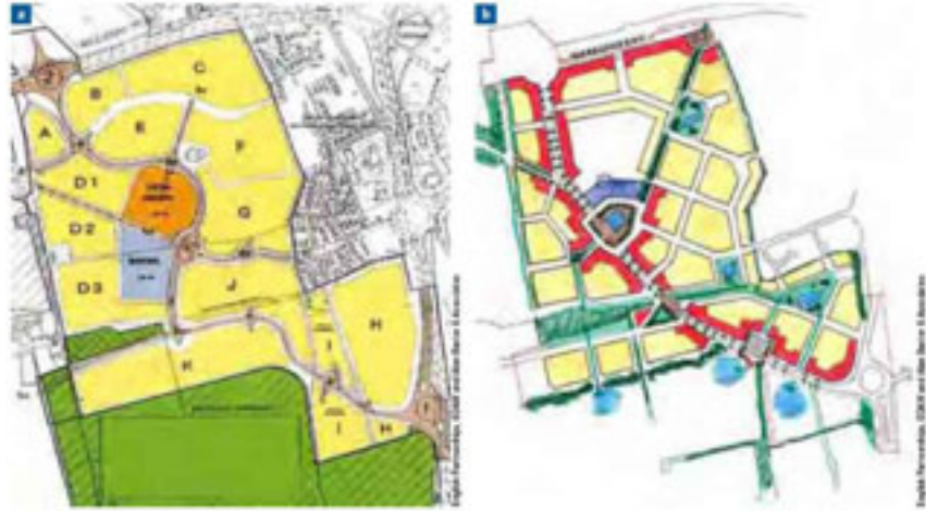
Figure G1.12 Alternative proposals for a development: (a) is roads-led; while (b) is more attuned to pedestrian activity and a sense of place.
