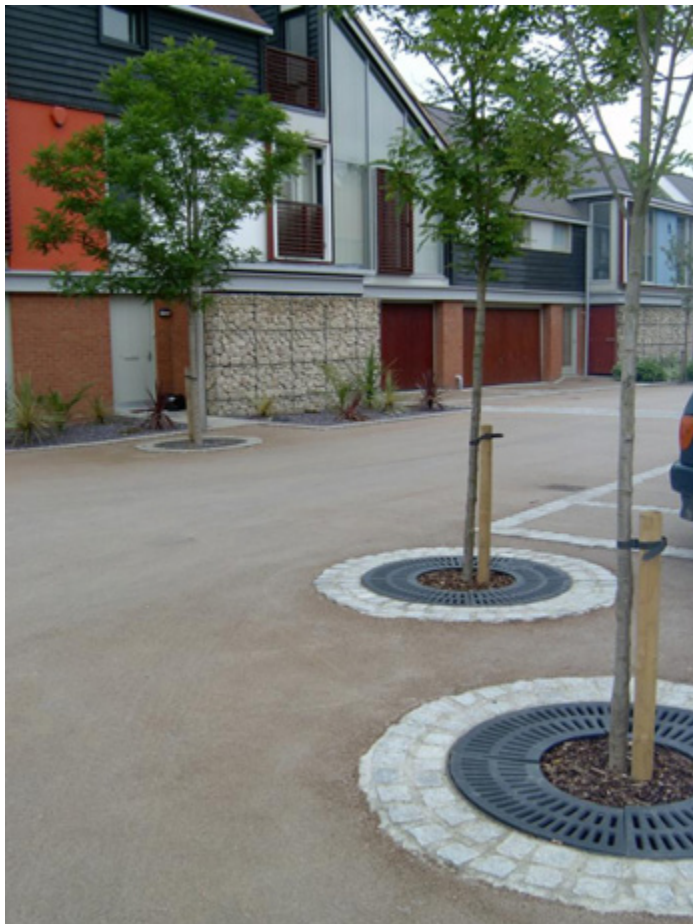
Figure G4.14 Trees planted in the highway at Newhall, Harlow, help to reduce vehicle speeds (EDAW).
