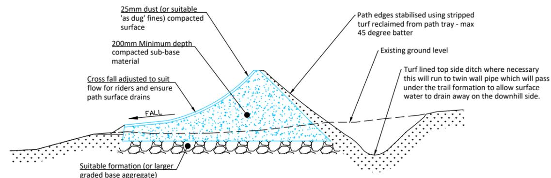
**Typical 'Berm' Trail Construction Detail**
