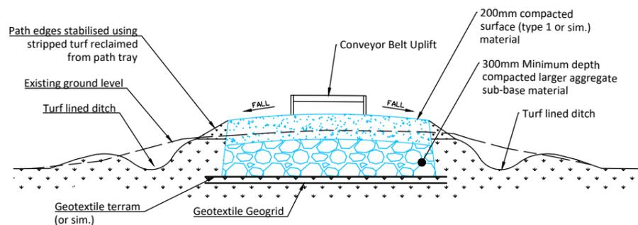
**Conveyor Belt Track Construction Detail**
