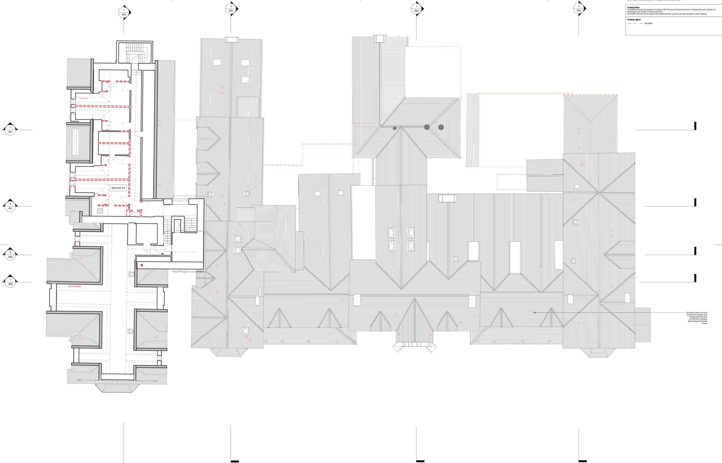
All existing cowls and vents removed and replaced with heritage style lead vents, and discreet ventilation grills existing penetrations re-used
