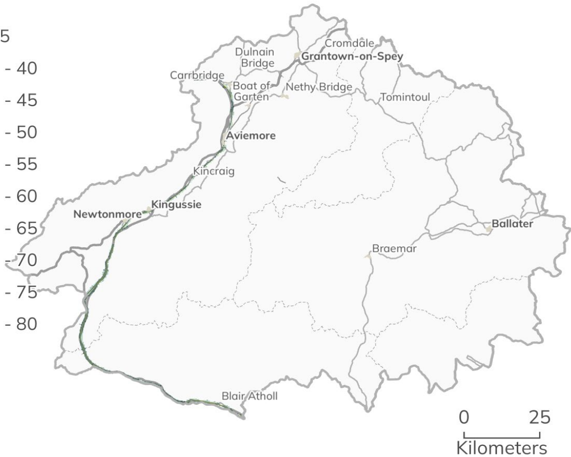
Figure 49 Noise from rail traffic - Map showing the day evening night level (Lden) noise indicator for overall annoyance based upon annual average A-weighted long term sound over 24 hours, with a 5dB(A) penalty for evening noise (19:00 – 23 :00) and a 10 dB(A) penalty for night time noise (23:00 – 07:00) attributed to rail use. Cairngorms National Park Authority © Crown copyright and database rights 2026 Ordnance Survey AC0000821810. Contains data © Scotland's noise, 2026 (CNPA1086).
