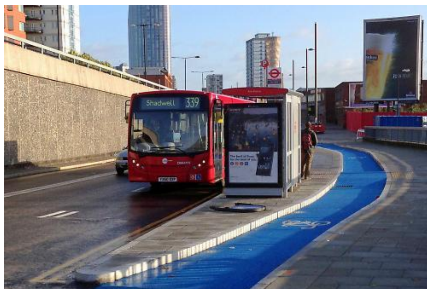
Figure 33: Floating Bus Stop Design
