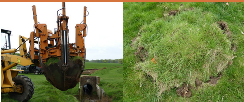
Moving a Yellow Meadow Ant nest using a tree spade. Image on left shows nest being carried by a compact loader equipped with a tree spade. Image on right shows nest once deposited by tree spade.
